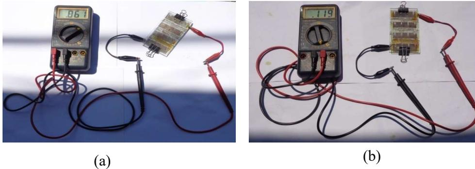
**Figure 17 (a)** The open circuit voltage  $V_{oc}$  **(b)** The short circuit current  $I_{sc}$  for four cells meander type DSSC module
