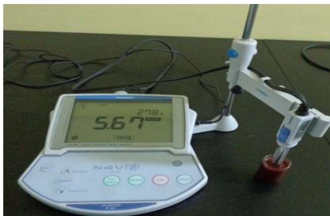
**Figure 12.** Measuring pH for teak leaves dye solution with pH meter
