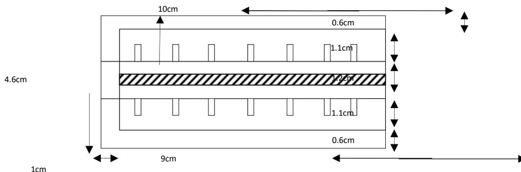
Figure 3(a) The design of TiO<sub>2</sub> electrode for two cells
