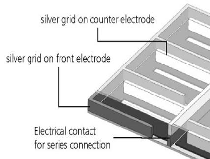
**Figure 1(c).** Aligning front and counter electrode on top of each other
