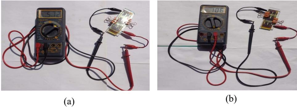
**Figure 16 (a)** The open circuit voltage  $V_{oc}$  (b) The short circuit current  $I_{sc}$  for three cells meander type DSSC module
