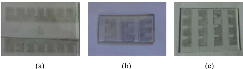
**Figure 8.** Carbon-coated counter electrodes for two cells, three cells and four cells
