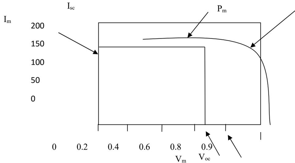
Figure 15. Current-voltage curve of a typical solar cell
