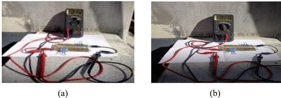
Figure 14 (a) The open circuit voltage  $V_{oc}$  (b) The short circuit current  $I_{sc}$  for two cells meander type DSSC module
