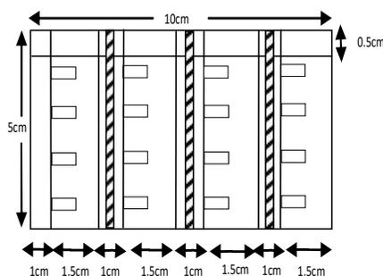
Figure 3(c). The design of TiO<sub>2</sub> electrode for four cells
