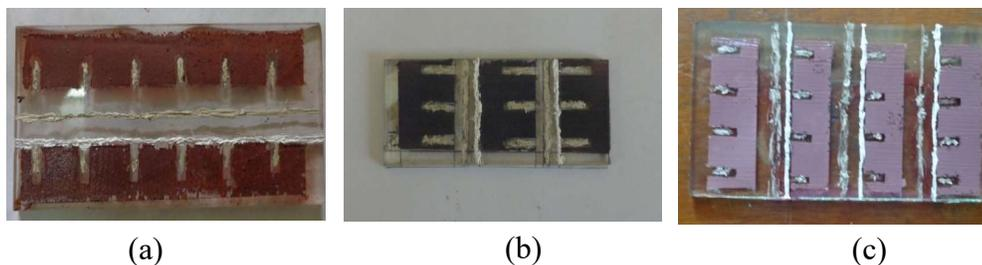
**Figure 9.** Drawing the silver lines and silicone on the  $\text{TiO}_2$  substrate for two cells, three cells and four cells
