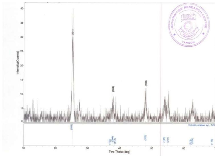
**Figure 11.** XRD pattern of TiO<sub>2</sub> nano-powder
