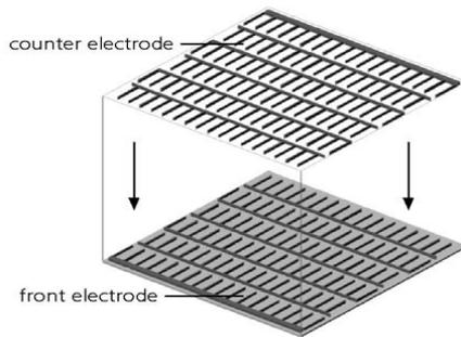
**Figure 1(b).** Front and counter electrode of a meander type DSSC module
