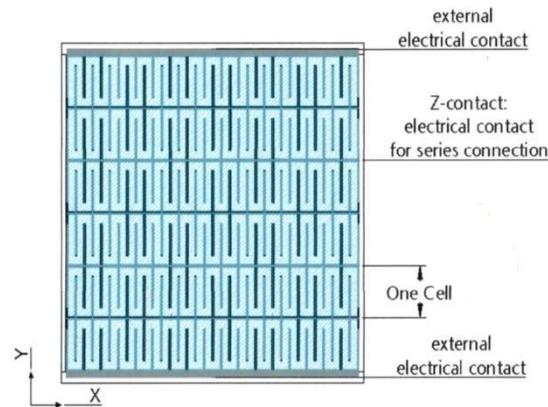
**Figure 1(a)** A meander type dye-sensitized solar cell module design
