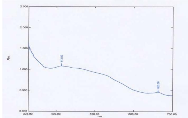
**Figure 13.** UV-Vis absorption spectra of liquid dye extracting with acetone from teak leaves
