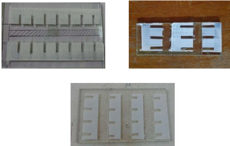
**Figure 5(a)**  $\text{TiO}_2$  coated plates for two cells, three cells and four cells
