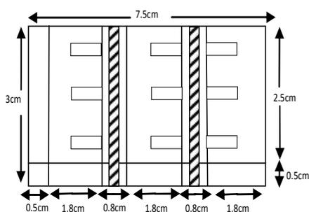
Figure 3(b). The design of TiO<sub>2</sub> electrode for three cells
