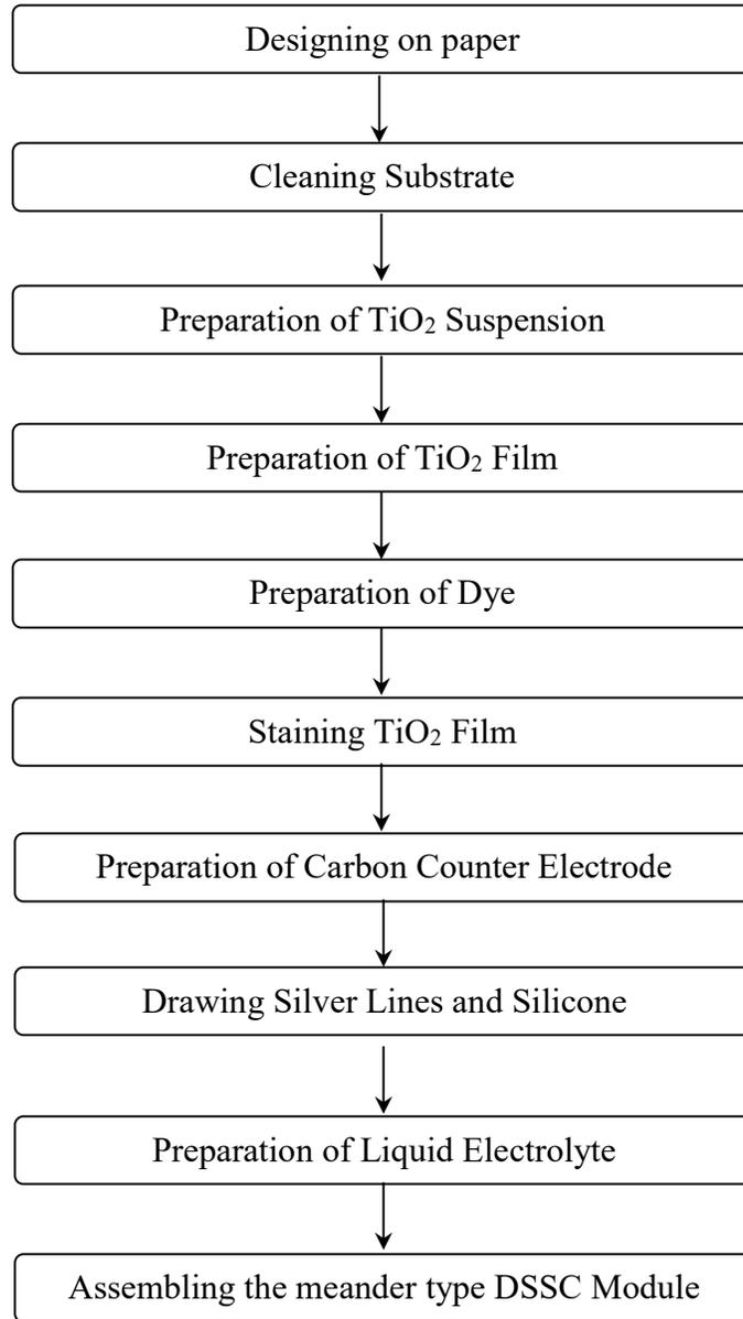
**Figure 2.** Flow chart for experimental procedures of meander type DSSC modules
